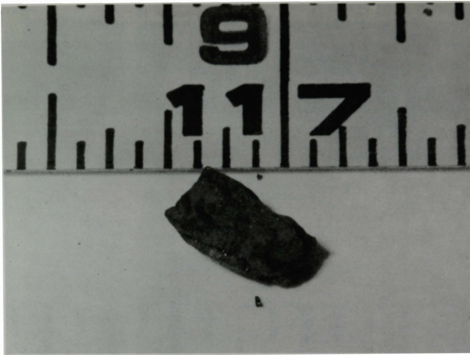
Figure 16. Particle 4-1, removed from TMI-2 core debris sample #4 (surface-E9).
