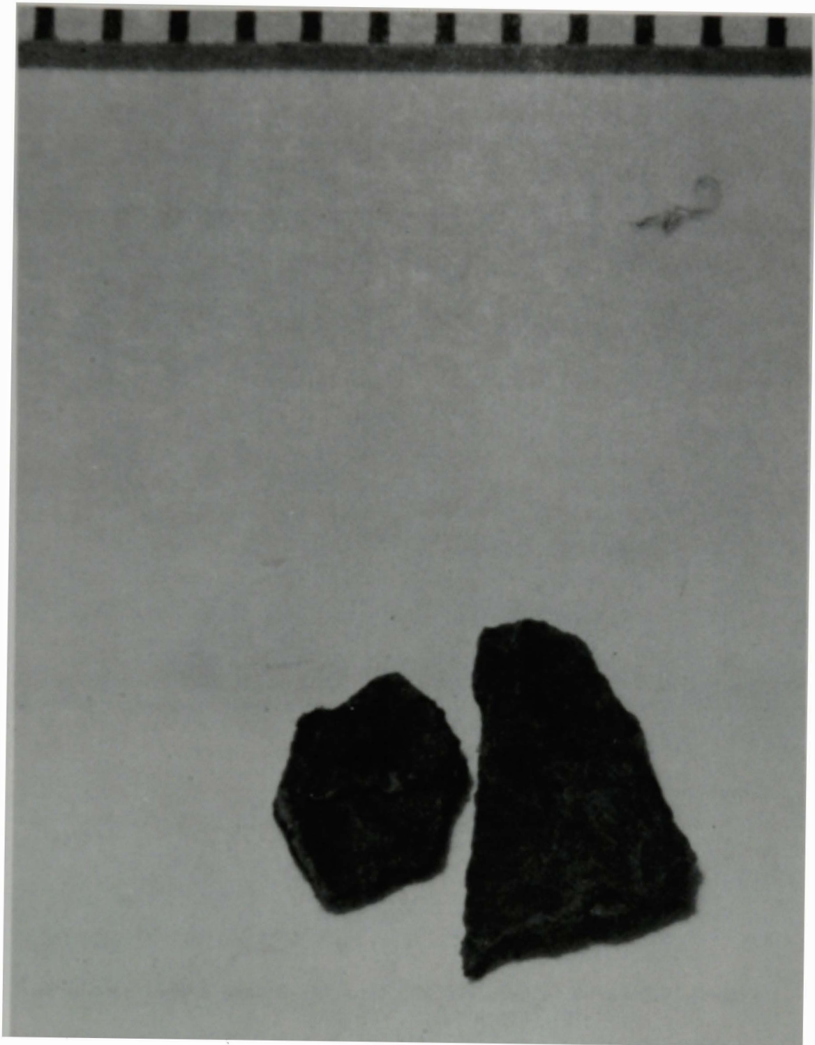
Figure 18. Particle 6-1, removed from TMI-2 core debris sample #6 (22 in. deep-E9).
